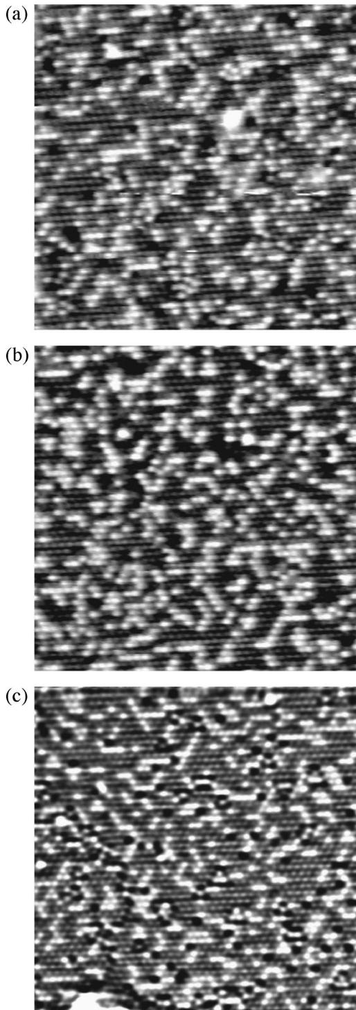
FIG. 4. STM images of (a) the surface formed by 25 min of HBO<sub>2</sub> irradiation ( $V_s=2.0$  V,  $I_t=0.8$  nA, 30 nm×30 nm), (b) the surface after annealing (a) at 750 °C for 5 min ( $V_s=2.0$  V,  $I_t=0.87$  nA, 30 nm×30 nm), and (c) the surface after annealing (b) at 900 °C for 8 s ( $V_s=2.0$  V,  $I_t=1.0$  nA, 30 nm×30 nm).
