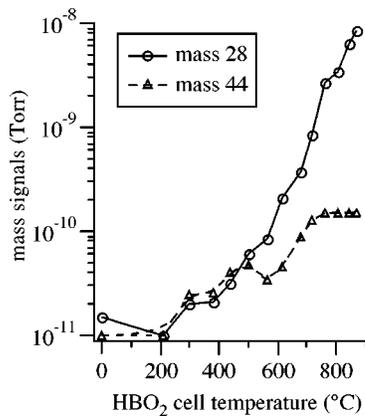
FIG. 2. Temperature dependence of mass signal from HBO<sub>2</sub> source.
