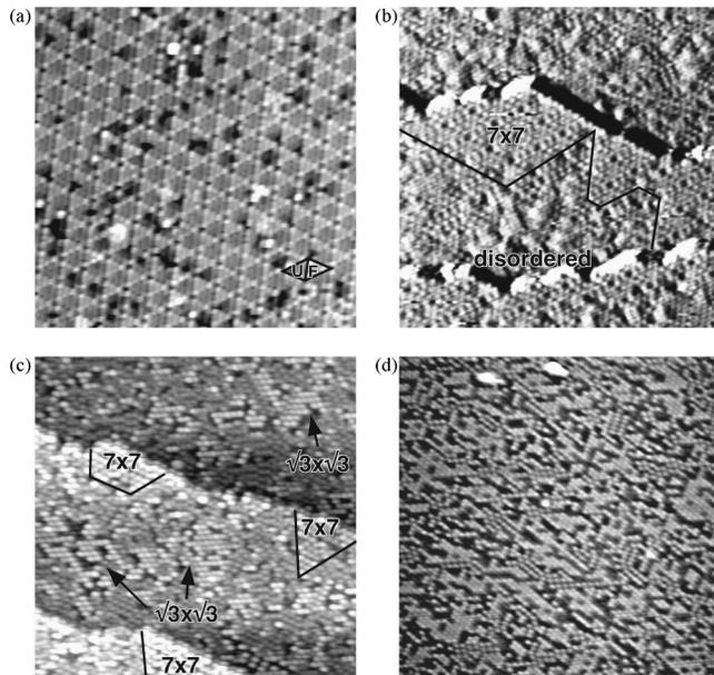
FIG. 1. STM images of the surfaces formed by (a) 3, (b) 5, (c) 6, and (d) 15 min of HBO<sub>2</sub> irradiation. Tip bias voltage  $V_s$ , tunneling current  $I_t$ , and scan size are (a)  $-2.0$  V,  $0.4$  nA,  $35$  nm $\times$  $35$  nm, (b)  $2.6$  V,  $0.4$  nA,  $35$  nm $\times$  $35$  nm, (c)  $-3.0$  V,  $0.33$  nA,  $35$  nm $\times$  $35$  nm, and (d)  $1.0$  V,  $1.0$  nA,  $35$  nm $\times$  $35$  nm, respectively.
